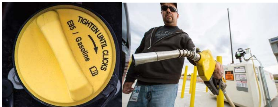
Figure 4. Yellow gas-tank cap of an FFV and matching dispenser nozzle
